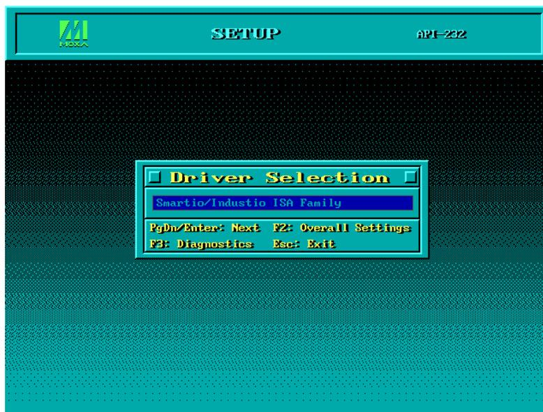
2. Press **Enter** to pop up the SETUP dialog box. In the SETUP dialog box, Press **F8** to specify the **CAP Address** and press **ENTER** and then type **Y (YES)** to load the configuration of the board to be setup.
