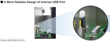
The Matrix internal USB 2.0 port provides increased application security with connectivity for license keys or password encryption on USB dongle.
