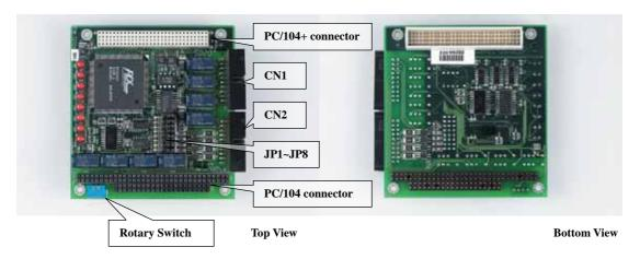
Figure 2 PCM-7250+ module layout
