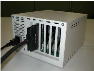
Figure 2.9. Plugging the power cable into the ECH(PCI)BE-H4A
