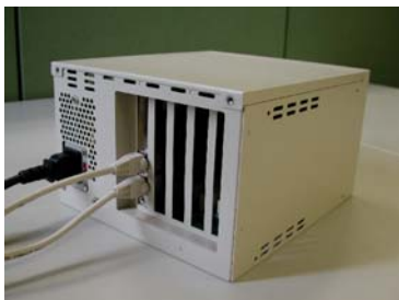
Figure 2.10. Plugging the power cable into the ECH(PCI)SF-H4A/H7A/F7A/H13A/F13A
