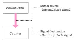
This example does not require any setup of the event controller for analog output. Event controller setup is only needed for the counter.
