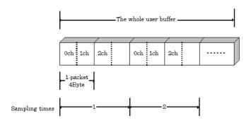
The figure above shows how data is transferred to the user buffer for the case when three channels (0ch, 1ch, and 2ch) are used.
