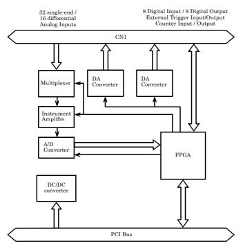
Figure 6.1. Block Diagram
