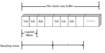
The figure above shows how to set the data in the user buffer for the case when three channels (0ch, 1ch, and 2ch) are used.
