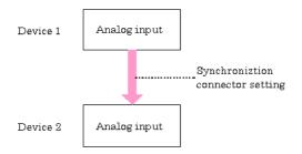
Synchronizing between two devices is performed by connecting control signals from device 1 to device 2.
