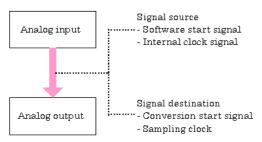
First, the conversion start signal for analog input can be configured to be used as the start signal for analog output so that analog input and output start simultaneously.
