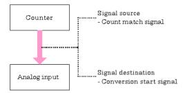
Connect the count match signal from the counter to the conversion start signal for analog input.
