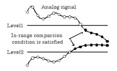
Start condition : Level 2 ≤ Analog signal ≤ Level 1
