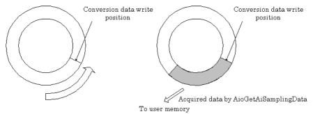
When using a user buffer, the conversion data is transferred directly to application memory by the driver.
