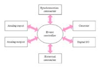
The arrows in the figure indicate the flow of control signals. The main control signals included clock signals and the operation start and stop signals.
