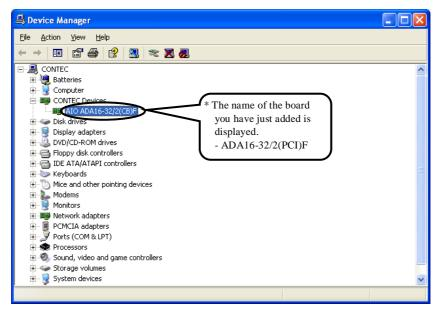
(2) The installed hardware appears under the CONTEC Devices node. Open the CONTEC Devices node and select the device you want to setup (the device name should appear highlighted). Click [Properties].
