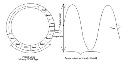
\* Although the figure shows a single analog output channel, output from multiple channels is also possible.
