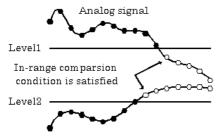
Start condition : Level  $2 \le$  Analog signal  $\le$  Level 1
