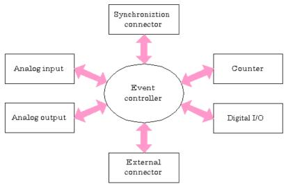
The arrows in the figure show the flow of control signals.
