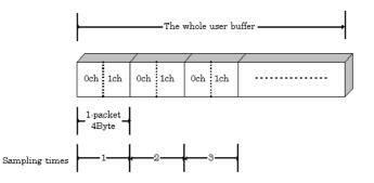
The figure above shows how data is transferred to the user buffer for the case when two channels (0ch and 1ch) are used. Data transfer uses a single 4 byte packet which is the minimum data transfer size. Each packet contains two AD conversion data values in binary format.
