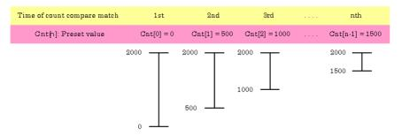
The figure above shows an example of using the preset value load function. In this example, the compare match value is set constant at 2000.
