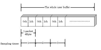
The figure above shows how to set the data in the user buffer for the case when two channels (0ch and 1ch) are used.
