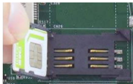
Insert Mini-SIM card with pins facing up
