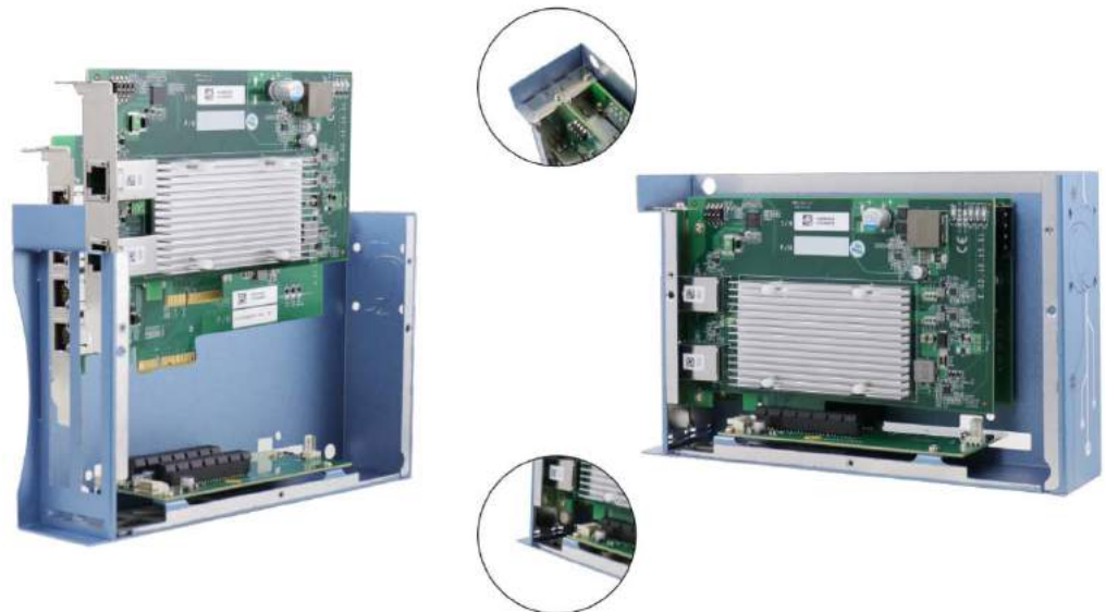
Nuvo-7000DE systems have two PCIe slots in the Cassette module
