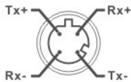
M12(4-pin, D-coding) Pin Assignments
