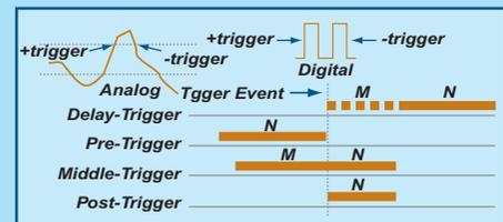
Pre-Trigger, Post-Trigger, Middle-Trigger, and Delay-Trigger. In addition, Post-trigger and Delay trigger modes allow successive triggers in order to capture repeated burst of data.
