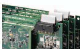
SSI bus cable for multiple cards synchronization
