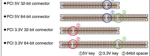
CONTEC provides 5V key-compliant boards supporting 5V PCI slots as well as universal key-complaint boards supporting both 5V and 3.3V PCI slots.
