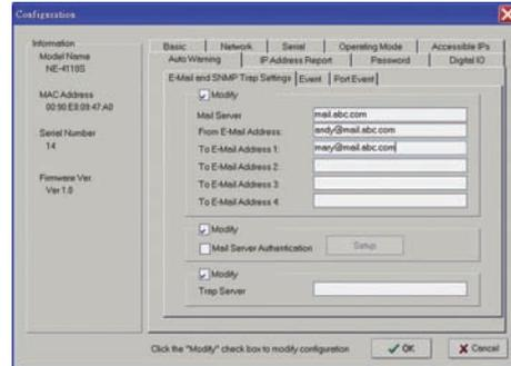
Remotely configure serial, network, alarm, and other parameters
