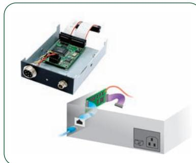
**NE-4120:** Pin-header Ethernet in stand-alone form factor
